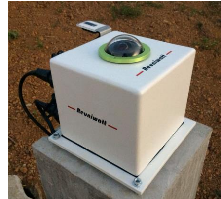
The Sky Cam Vision™ sky imager as installed at two locations in Morocco.
