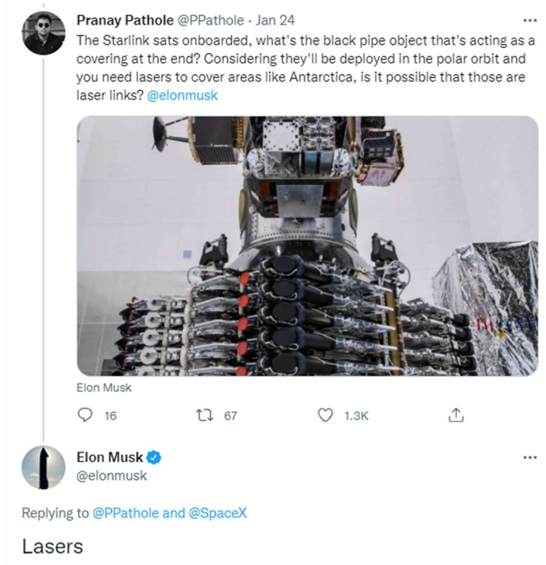
Figure 5 - A batch of Starlink satellites readied for launch in January 2021 that were confirmed to be equipped with inter-satellite optical links. (Image credits: Pranay Pathole at Twitter)
