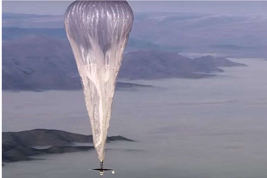
Figure 4 – One of Google Loon’s early test flights with the laser communications payload located on the platform below the balloon. (Image credits: Google)
