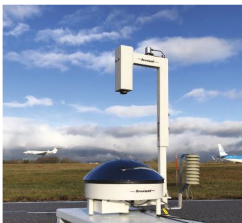
ABOVE: Figure 2 – Sky InSight is the first all-sky imager to use an infrared camera for observing the atmosphere both day and night
